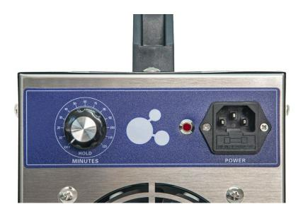
Fuse: A replaceable fuse (3A) is located beside the power supply.
